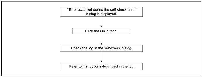
Figure 6.2 Flowchart to check the self-check error
